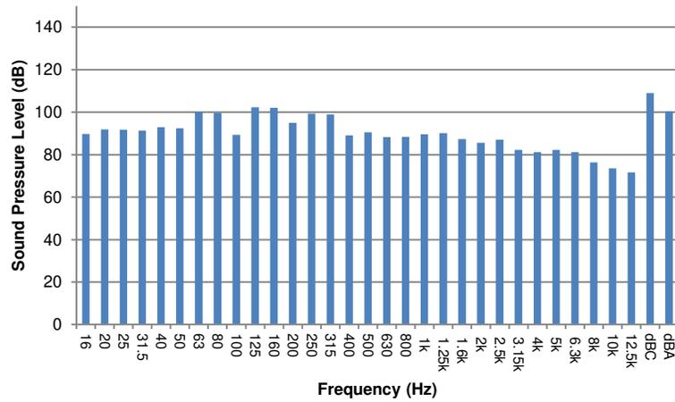
The installation of the custom noise abatement equipment resulted in a total reduction in sound pressure levels of approximately 27.9 dBA and 41.6 dBC.
