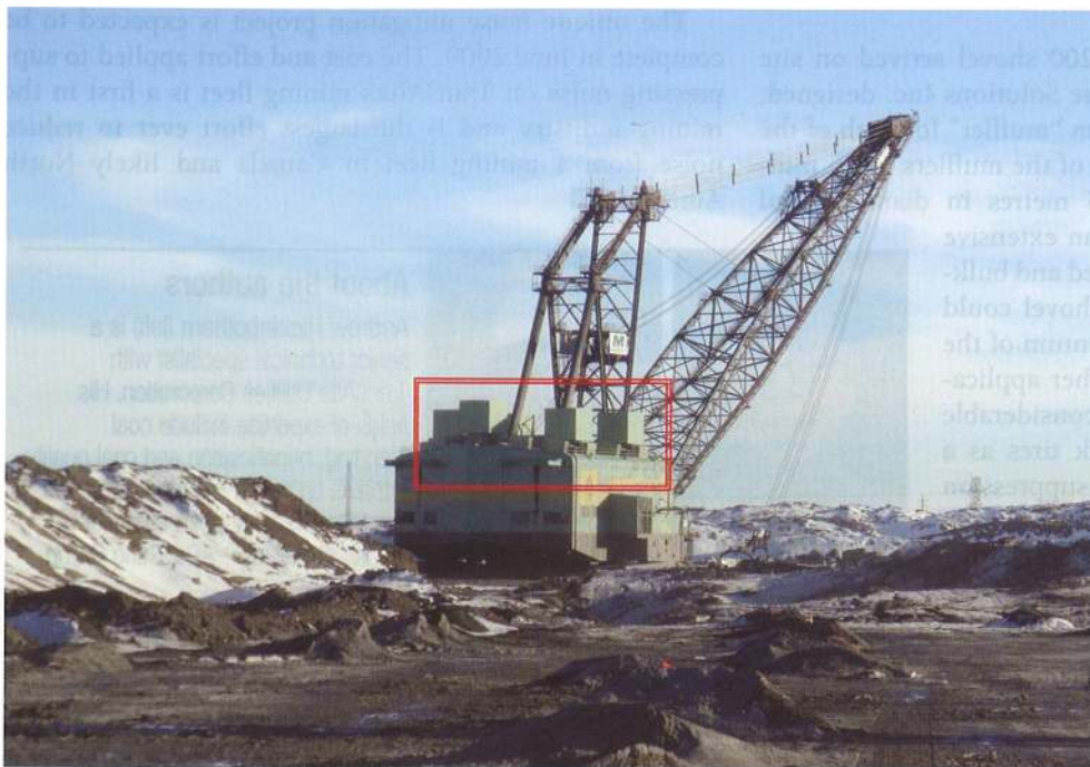
Fan hood on the Marion 8750 dragline helps suppress noise.
