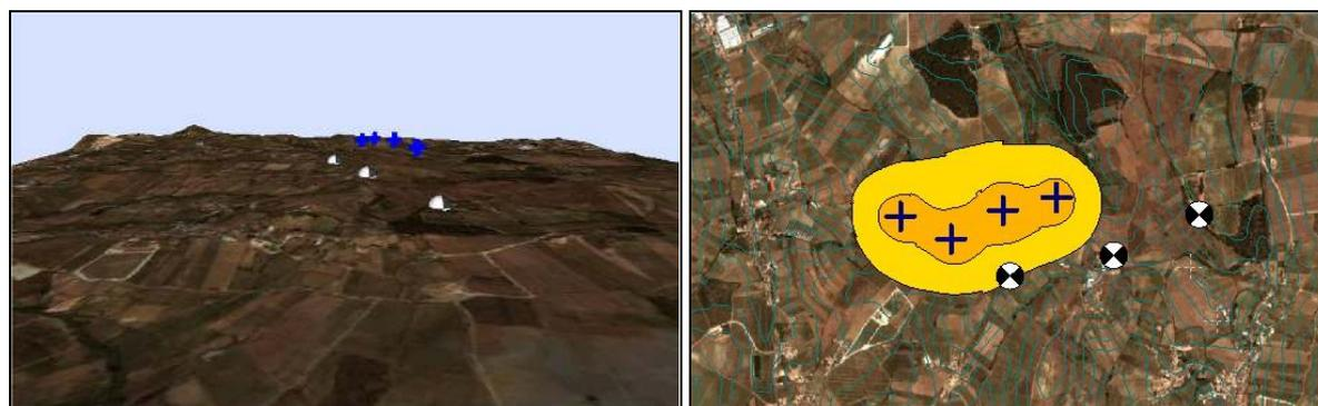
Figure 14 – 3D view of the model (left), showing a superposition of the orthophoto onto the terrain; and noise map in terms of  $L_{den}$  (right) .
