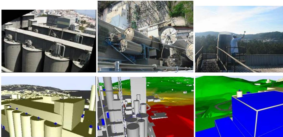
Figure 5 – Examples of sources modelled as (from left to right): point sources – fans on top of deposits, chimneys; line sources – high pressure pellets transportation pipes; plane sources – light metal façades and roof, openings.
