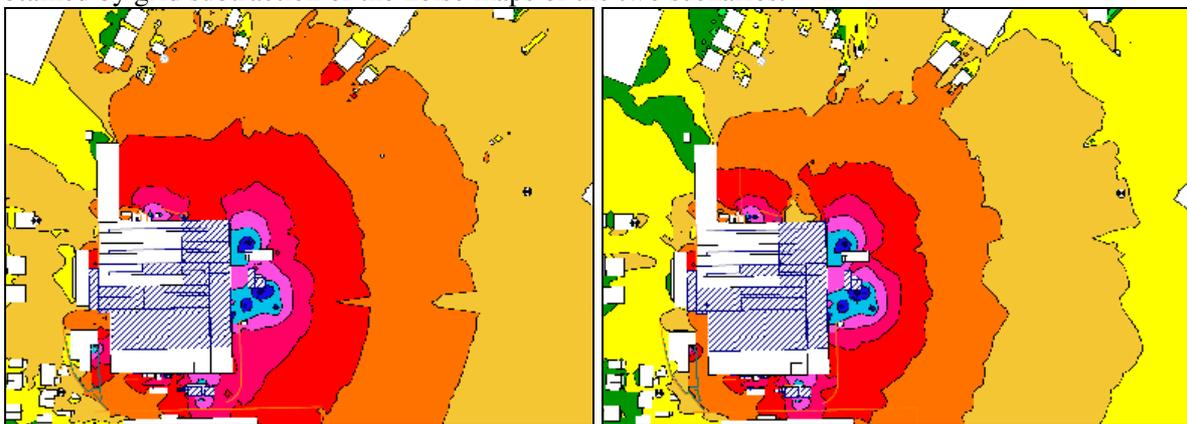
Figure 10 – Noise maps of the foundry after the expansion without (left) and with (right) noise control measures.
