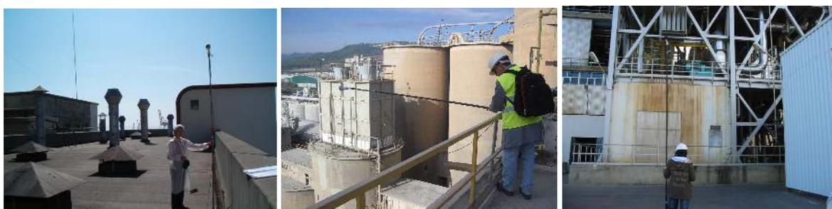
Figure 3 – Source validation: measurements within the factory but not too close to the sources.
